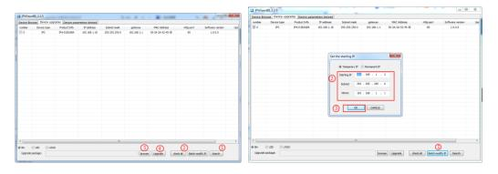
Step 2: For multi-devices batch upgrade, user need to modify the default IP address to different one to avoid IP address collision. Take an example as below pic shows:
